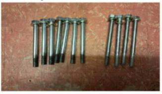
New head gasket fitted to block using 2 of the old studs as guides. Studs then removed and the new bolts with washers fitted and torqued down starting at 20 psi and working up to 35 psi in 5 psi increments.
