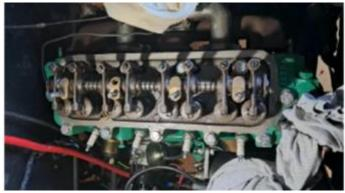
Head in place with rocker assembly and bolts torqued down.
