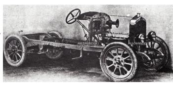
pension was semi elliptics at the front and cantilever at the rear. A test in 1922 gave 55—60 mpg and 25mph. It is likely that only 1 car was built.
