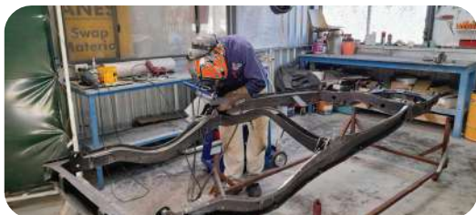
Joe Ciantar welding brackets to the Morris Z chassis for Jeff Cox
